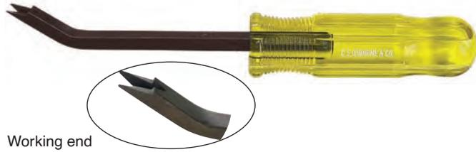
The correct angle for removing staples of any size, from the smallest to the longest leg staples. Manufactured from alloy tempered steel. Electronically hardened working ends. Fluted amber cellulose acetate handle to keep from rolling.
