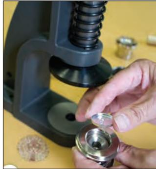
4.-Lay wire eye on the bottom die with the loop facing down.
