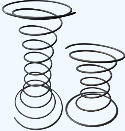
Open ended, 9 gauge. Upholstery springs are ideal for 8-way hand tied seating. Available in sizes from 5" to 10" height. Made of high carbon spring wire and heat treated for resilience. Sold in bundles of 25 lbs/ bundle. Data in table below is approximate and not exact.
