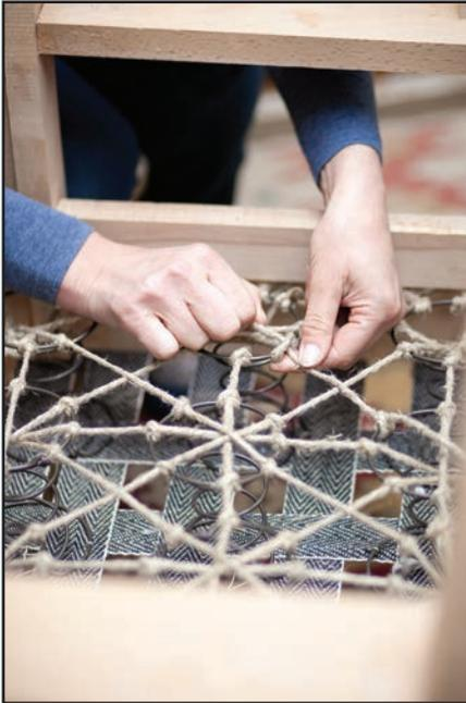
Italian made spring twine is the best in the industry. Our spring twine is made from the finest, strongest jute and is ideal for 8 way-hand tying of upholstery springs. Available in 1 lb. and 4.5 lbs. rolls.
