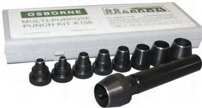
This handy and versatile kit contains threaded handle with self-centering pointed plunger. The threaded handle will accommodate nine interchangeable threaded cutting tubes. The punches in this set will cleanly cut leather, rubber, paper, plastics and other soft materials. The self-centering point makes these punches ideal for cutting concentric washers in small quantities by hand. Sizes of punches listed below. All cutting edges properly hardened. Comes in a sturdy plastic box for storage.
